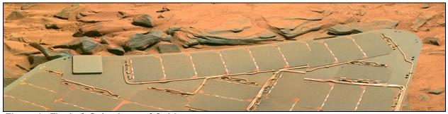
Figure 1. The Left Solar Array of Spirit
